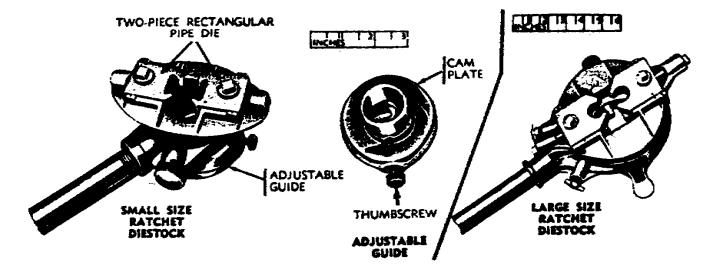
Figure 34. Adjustable die guide and ratchet diestocks.
