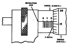
Figure 57. Reading standard micrometer scale.
