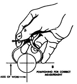
Figure 51. Using outside calipers.
