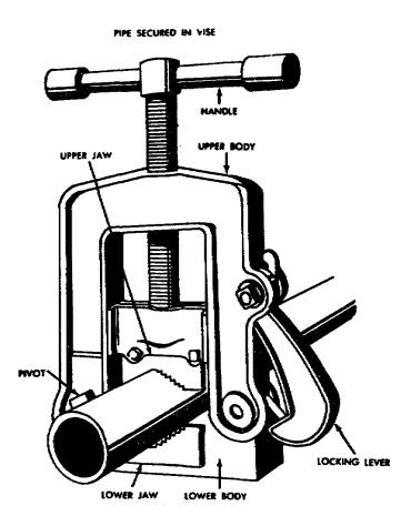
Figure 16. Pipe clamped in vise.
