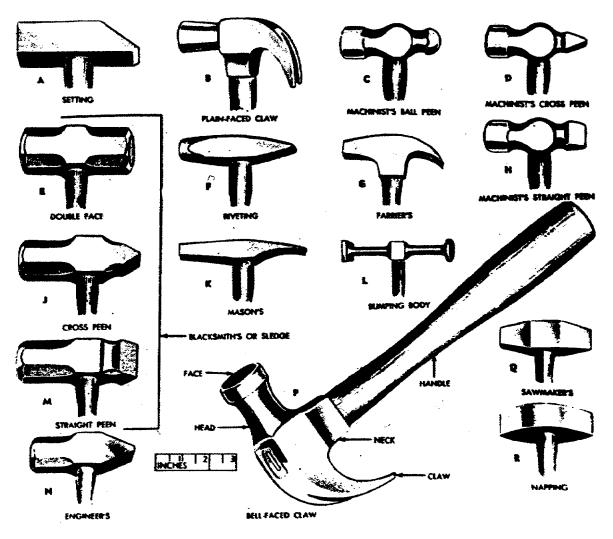
Figure 1. Types of hammers.
