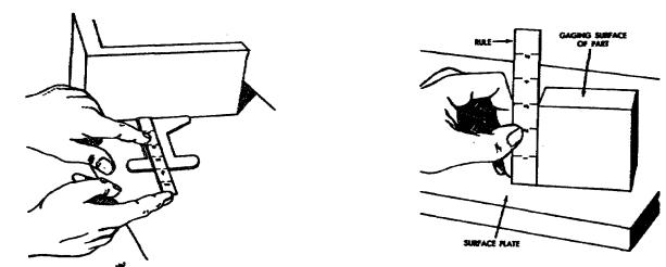
Figure 44. Using 6-inch rule. Figure 45. Using rule on surface plate.
