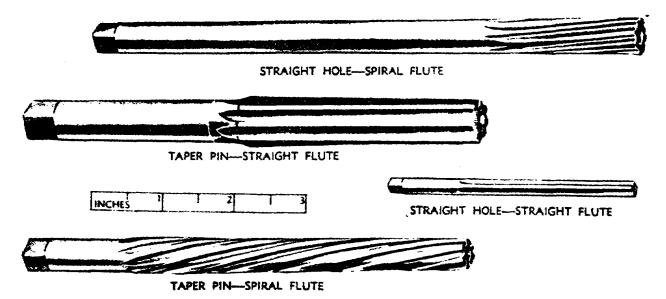
Figure 23. Solid straight hole and taper pin reamers.
