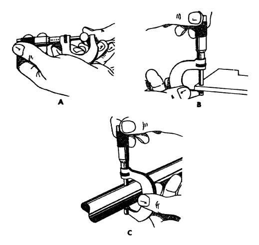
Figure 58. Using outside micrometer.
