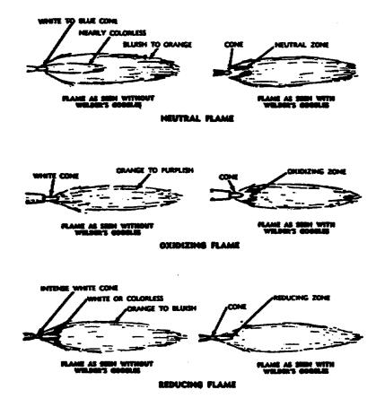
Figure 11. Oxyacetylene flames.
