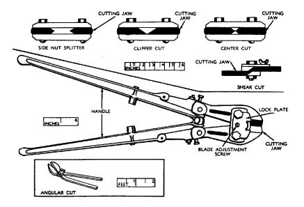
Figure 38. Types of bolt and nut cutters.
