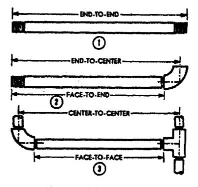
Figure 10. Threaded pipe measurements.
