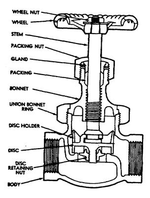
Figure 44. Details of globe valve.
