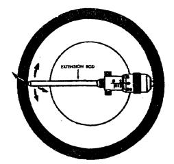
Figure 60. Using inside micrometer with extension rod.
