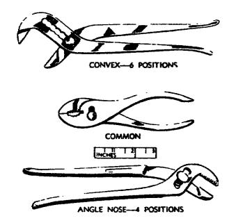
Figure 26. Slip joint combination pliers.
