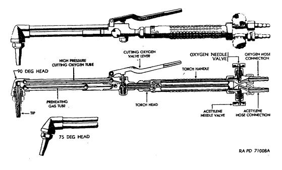
Figure 15. Cutting attachment for welding torch.
