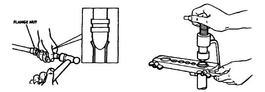
Figure 21. Using the flaring tool.
