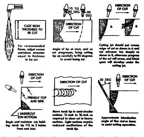
Figure 17. Procedure for oxyacetylene cutting of cast iron.
