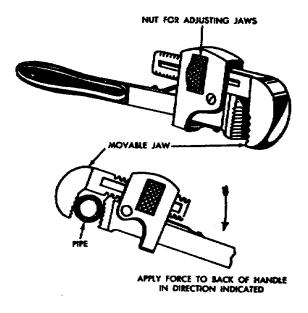
Figure 16. Using adjustable pipe wrench.
