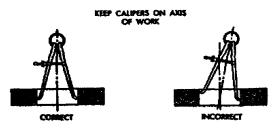
Figure 53. Positioning of inside calipers.
