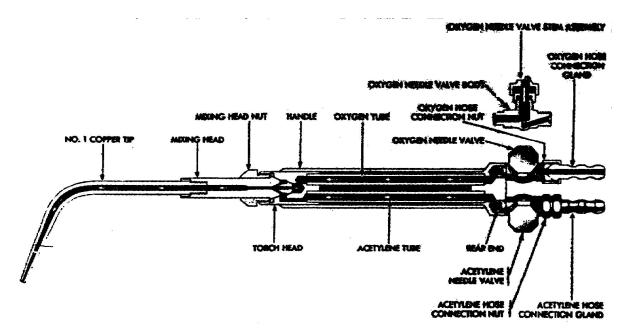
Figure 7. Equal pressure type, general purpose welding torch.
