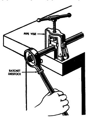
Figure 40. Threading pipe.
