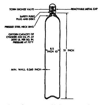
Figure 3. Oxygen cylinder construction.
