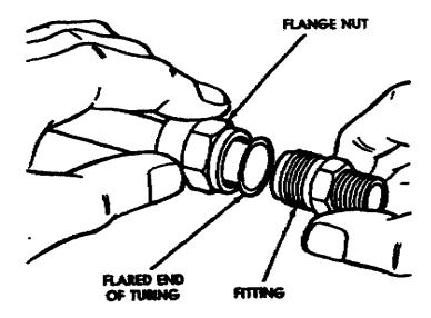
Figure 22. Making up a flared fitting.
