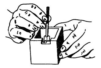
Figure 46. Using small rule and holder.
