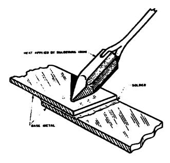
Figure 26. Method of sweating a lap-joint.
