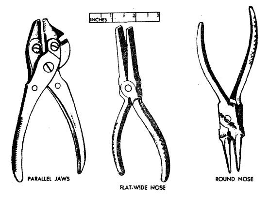
Figure 28. Parallel jaws, flat, and roundnose pliers.
