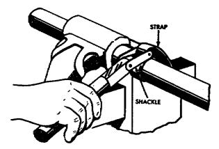
Figure 17. Using a strap pipe wrench.
