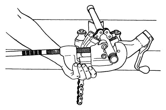
Figure 19. Cutting pipe.
