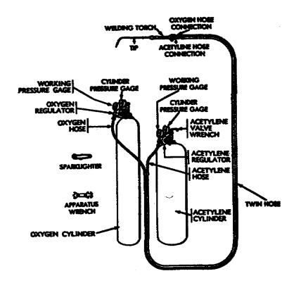
Figure 2,. Portable oxyacetylene welding equipment,
