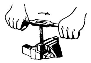
Figure 37. Using a tap and tap wrench.
