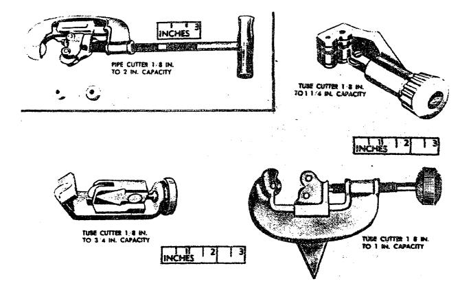
Figure 17. Pipe and tube cutters.
