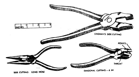
Figure 27. Diagonal and side cutting pliers.
