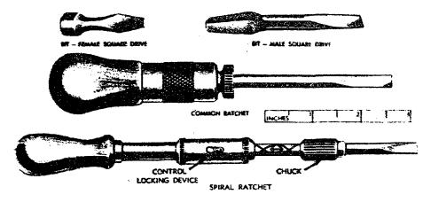
Figure 23. Ratchet screwdrivers and screwdriver bits.
