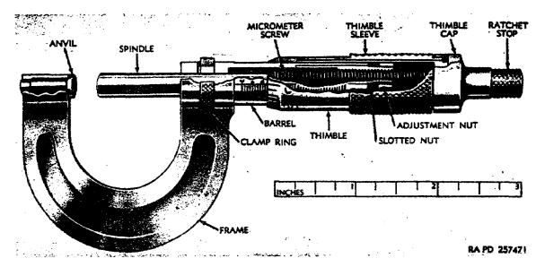
Figure 56. Micrometer, caliper, cutaway view.
