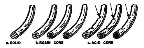
Figure 21. Forms of wire solder.
