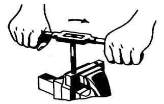
Figure 26. Reaming operation.
