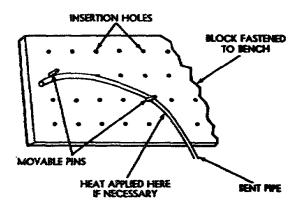
Figure 14. Bending block and pins.
