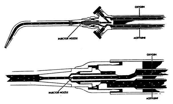
Figure 6. Mixing head for injector type welding torch.
