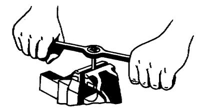
Figure 39. Using a die and diestock.
