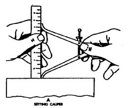
Figure 54. Using a transfer caliper to measure a recessed diameter.
