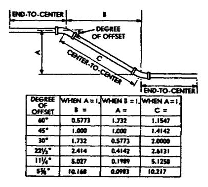
Figure 12. Pipe measurement for offsets.
