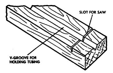
Figure 20. Jig for cutting tubing with a hacksaw.
