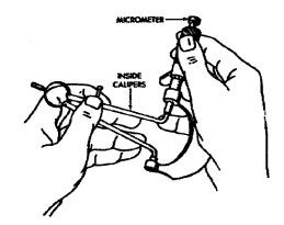
Figure 55. Transferring dimension to micrometer.
