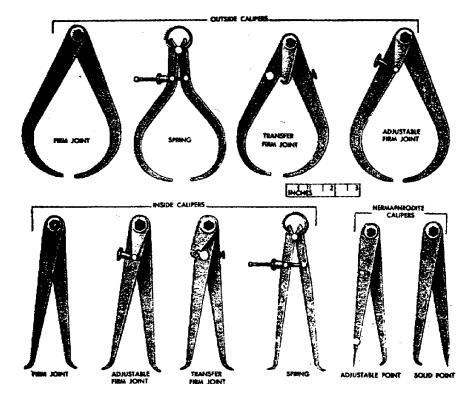
Figure 50. Calipers-noncalibrated.
