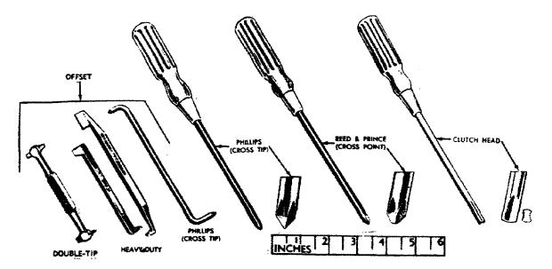
Figure 22. Special tipped screwdrivers.
