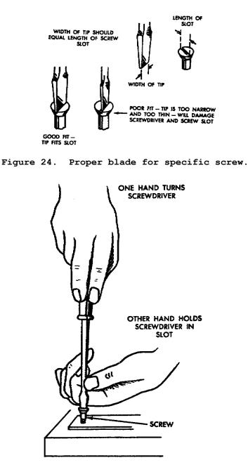
Figure 25. Holding screwdriver properly.
