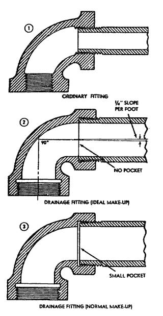
Figure 1. Difference between ordinary and drainage fittings.
