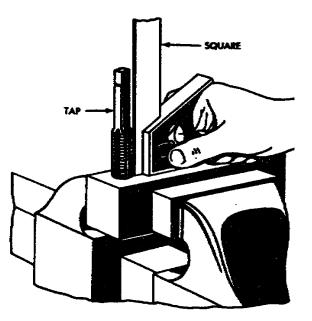
Figure 38. Checking tap for straightness.
