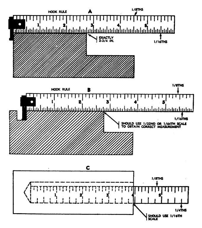
Figure 43. Determining proper graduated rule.
