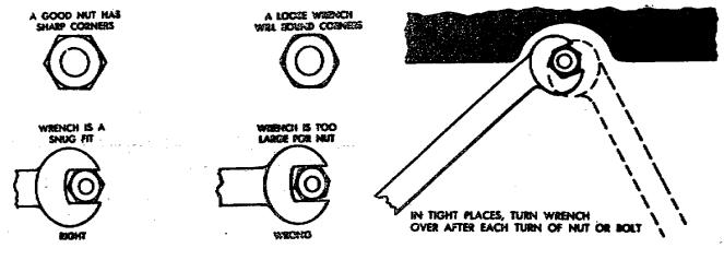
Figure 13. Fitting open end wrench.
