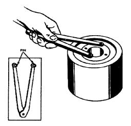
Figure 18. Using a pin-face spanner Figure 19. Using adjustable spanner wrench.
