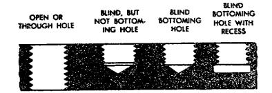
Figure 36. Types of drilled holes.
