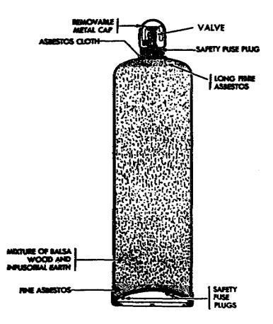
Figure 4. Acetylene cylinder construction.
