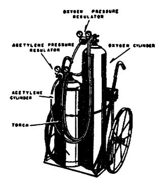
Figure 8. Complete truck, cylinders etc, with welding torch.
