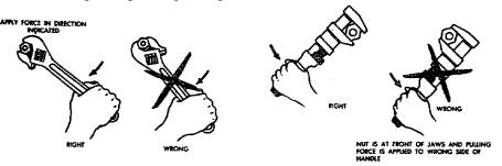
Figure 15. Using adjustable wrenches.
