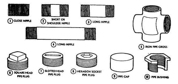
Figure 6. Miscellaneous iron pipe fittings.
