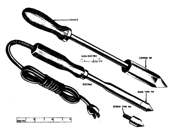
Figure 22. Soldering irons.
