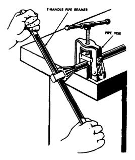
Figure 28. Removing bur from cut pipe.
